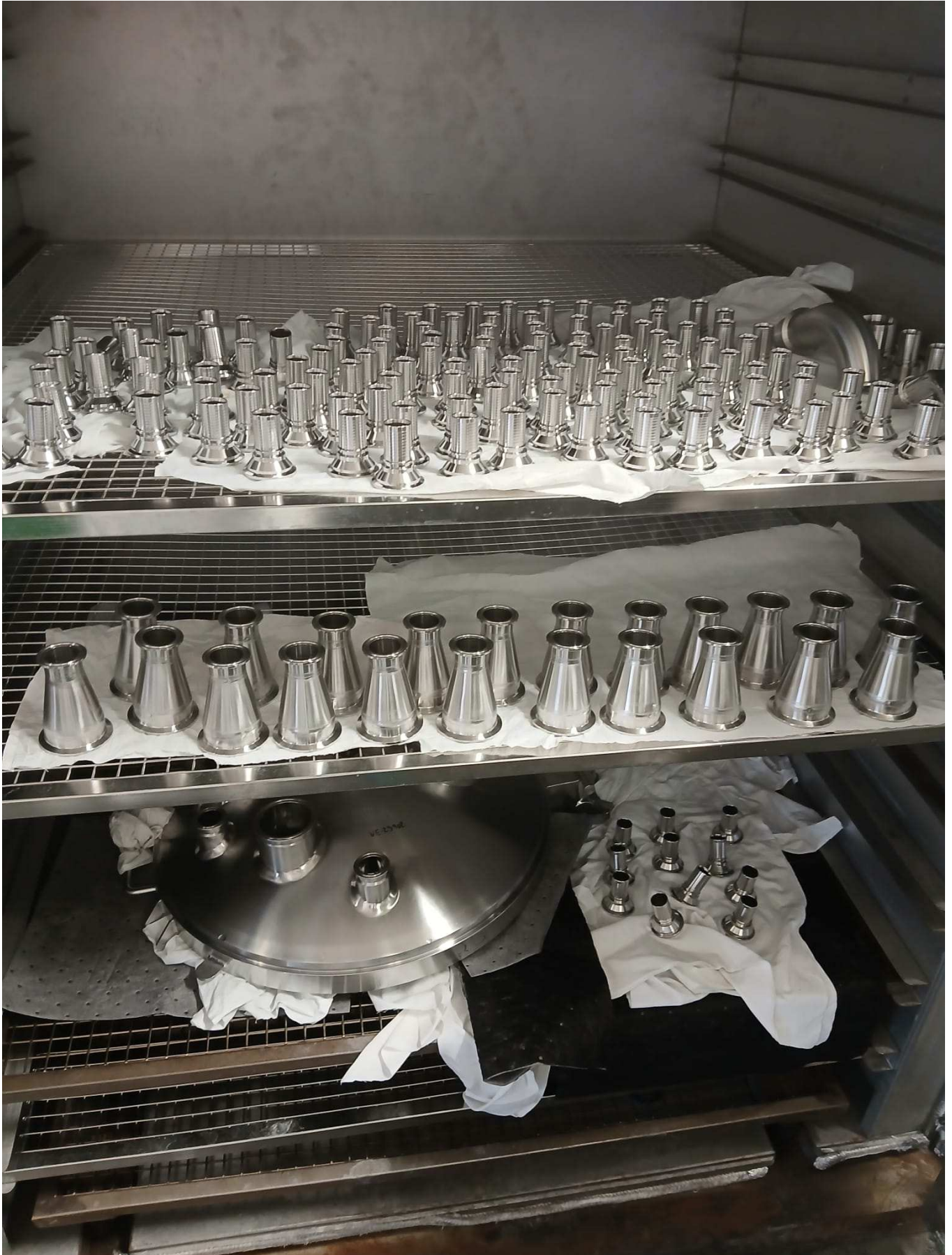
Parts in the oven after specialist cleaning and polishing.
